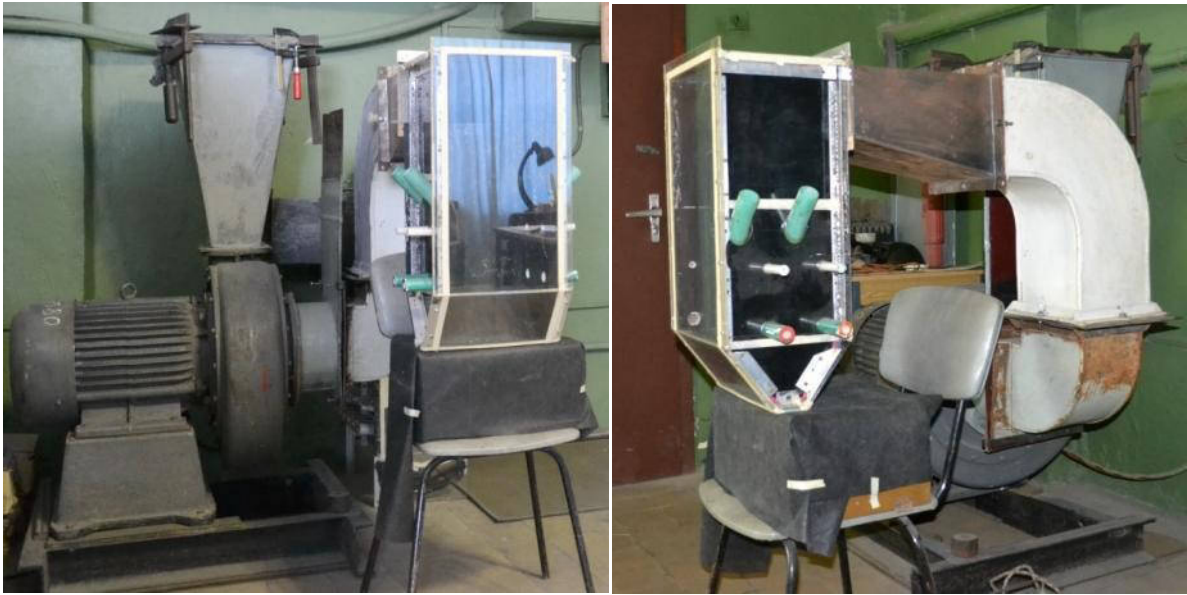
Fig. 4. General view of the experimental plant for studying the furnace aerodynamics at the boiler №2
