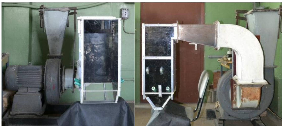
Fig. 15. General view of the test plant for studying furnace aerodynamic of the boiler №1.
