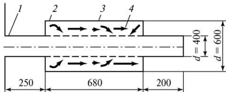
Fig. 5.53. Silencer for exhaust at Mutnovsky GeoPP: 1 — flange; 2 — casing; 3 — perforated outer surface; 4 — metal net
