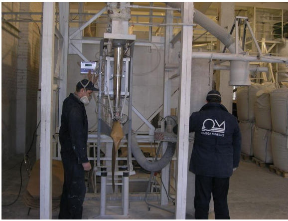
Fig. 5. Preparation for the shipment of hollow ash microspheres
