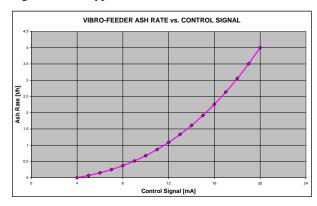
Fig. 4. Vibrofeeder ash rate vs. Control signal
