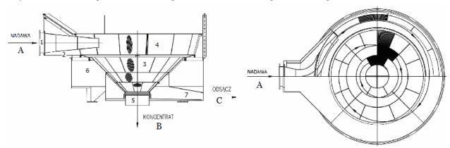
Fig. 1. Centrifugal dewatering sieve-OSO: A – feed material: B –concentrate; C –drain-off; 1 –nozzle outbox; 2 –steering wheel casing; 3 – conical sieve basket; 4 –steering wheel ; 5 –dewatered product exit; 6 –drain-off cumulative vessel; 7 – drain-off exitumption.
