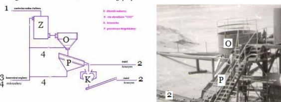
Fig. 2: A diagram of slag separation and dewatering and a picture of elporyt aggregate production system: 1 - feed material; 2 - slag/aggregate; 3 - coal concentrate + cenospheres; 4 - drain-off; Z - feeding tank; O - centrifugal sieve; P - screen; K - crusher
