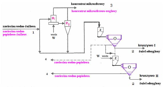
Fig. 3. Production of slag aggregates, coal concentrates, and cenospheres - a diagram
