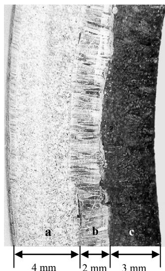
Fig. 1. The cross-section of steel pipe with aluminothermic coating: a – the pipe wall, b – an intermediate metal layer, c – ceramic layer.
