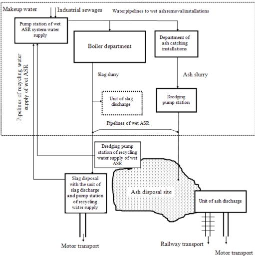
Fig. 2. Block diagram of wet ASR system with separate removal, landfilling and discharge of ash and slag.
