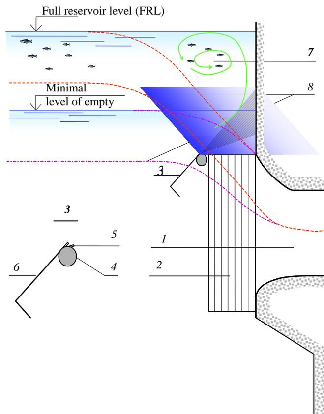
**Fig. 5.51. Using of water streams for fish protection at hydropower station:**
