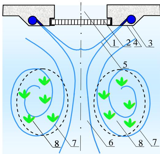
**Fig. 5.50. A layout of additional equipment of the universal fish-protection unit of "Volume hydraulic screen" type with fish-inhabited shelter**
