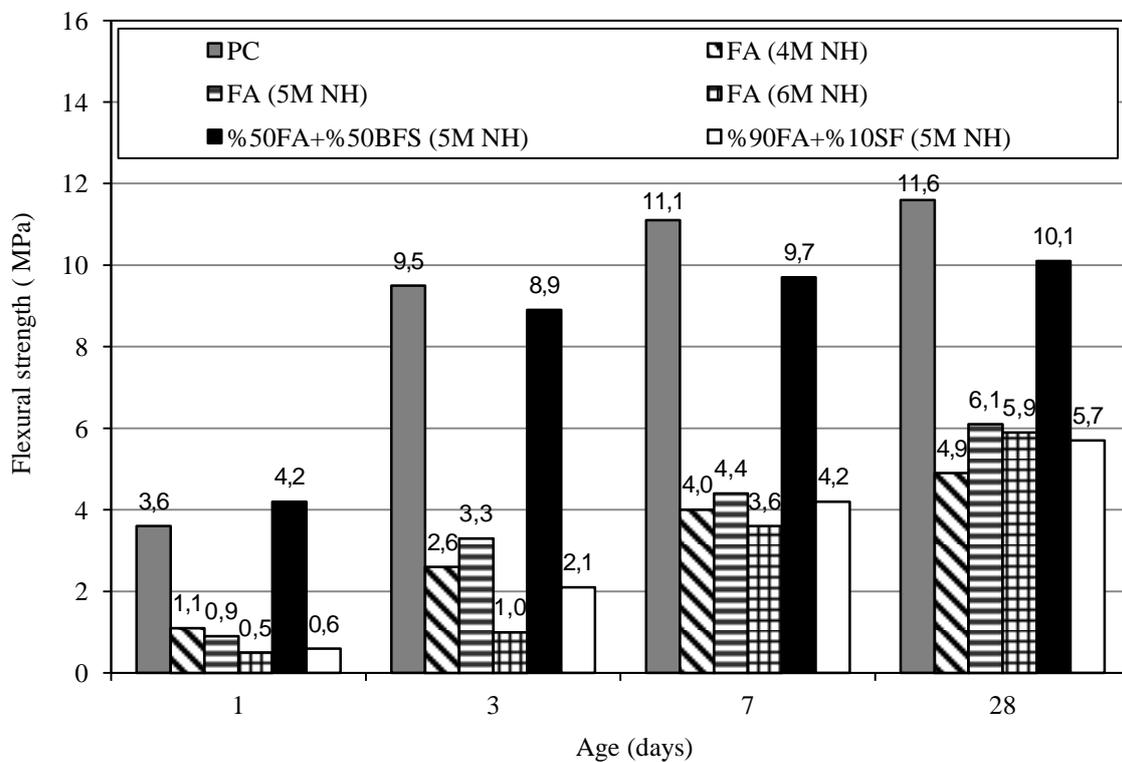
Fig. 3. Flexural strength of standard cured mortars
