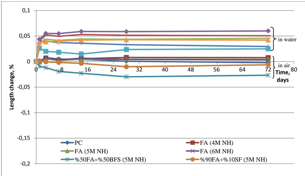
Fig. 8. Dimensional stability of autoclave cured mortars
