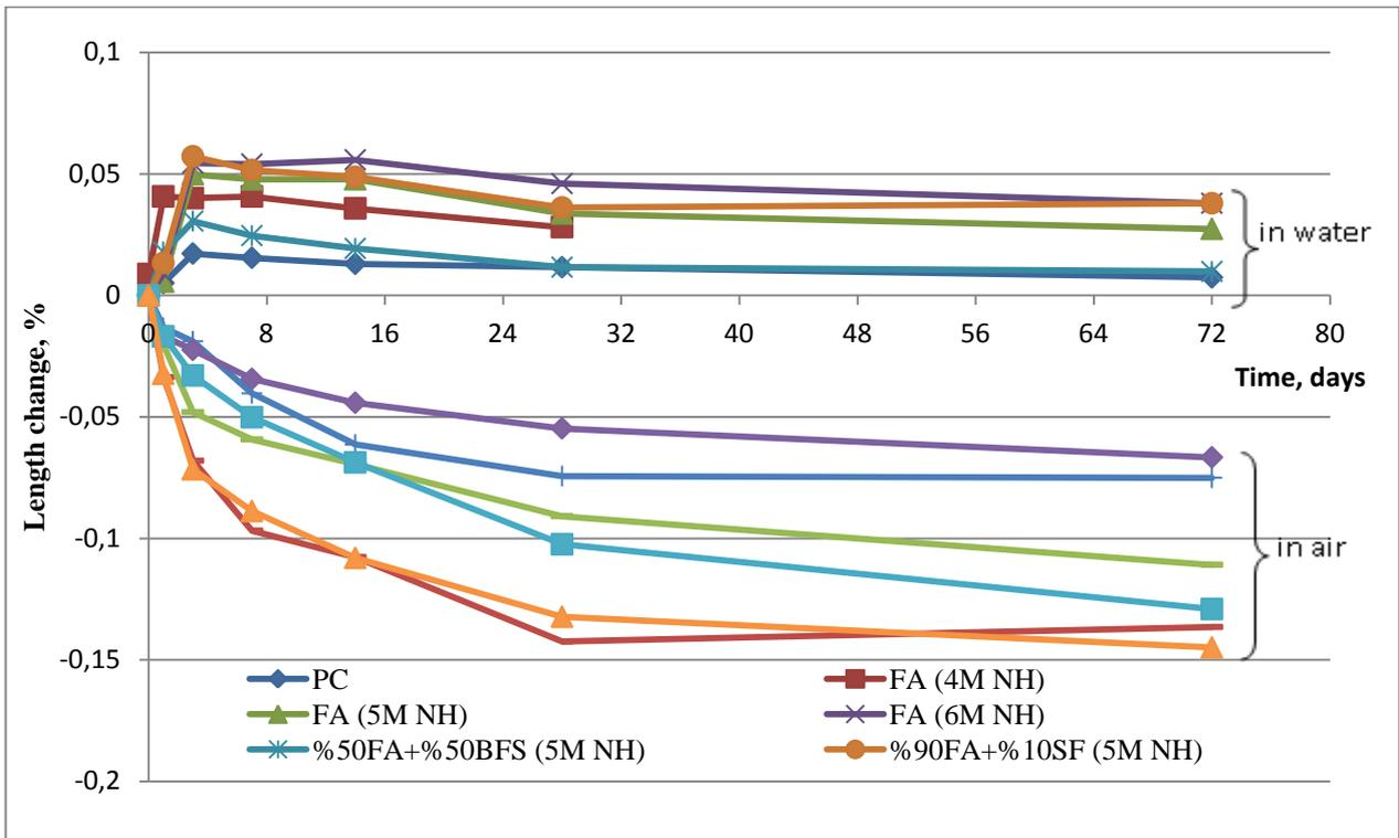
Fig. 6. Dimensional stability of standard cured mortars
