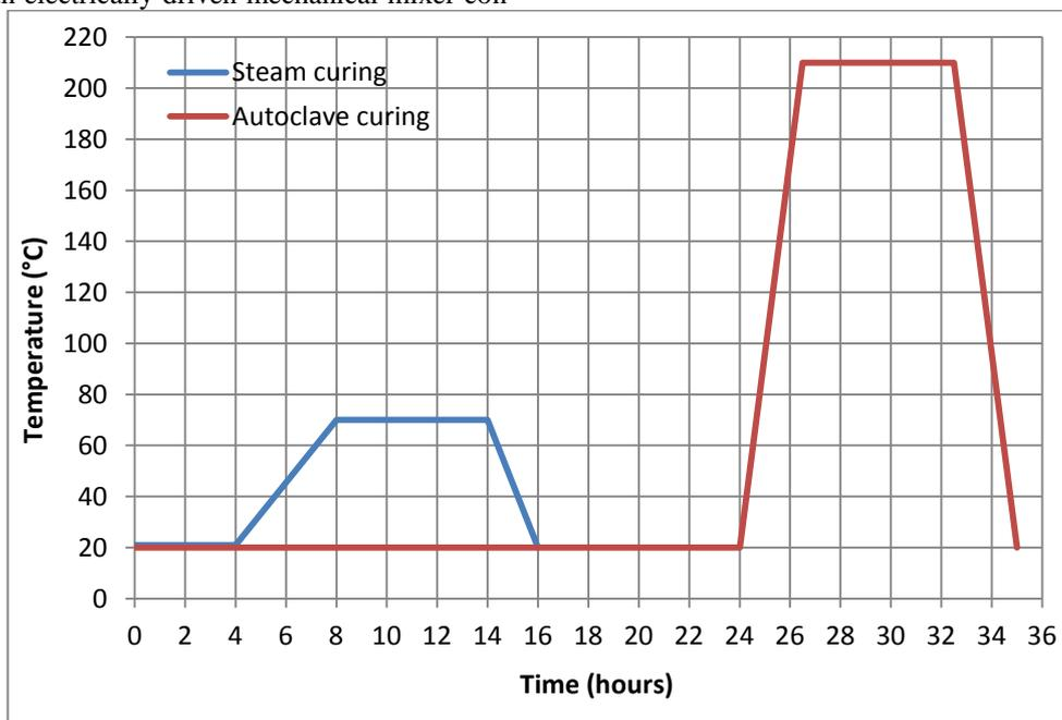
Fig. 1. Heat treatment cycles
