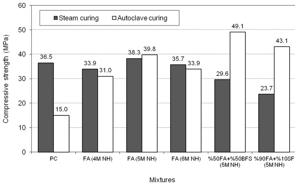
Fig. 4. Compressive strength of steam and autoclave cured mortars
