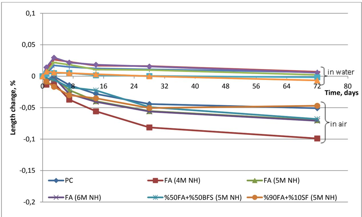
Fig. 7. Dimensional stability of steam cured mortars
