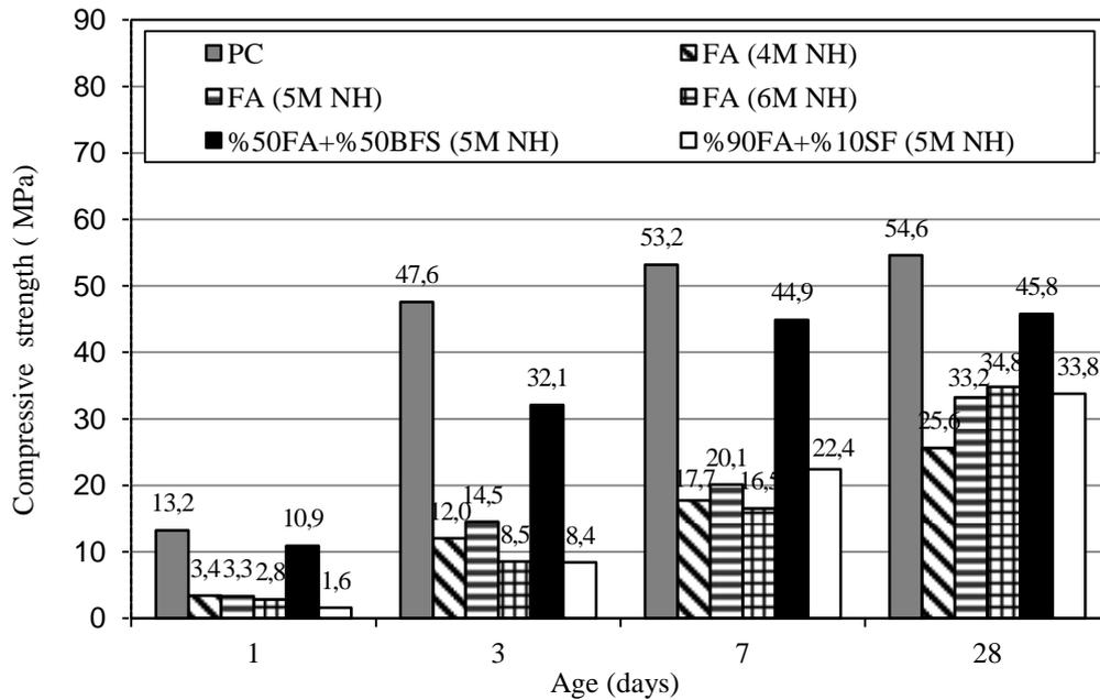
Fig. 2. Compressive strength of standard cured mortars
