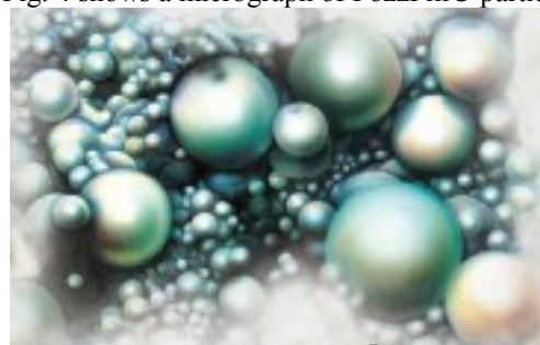
Fig.4. Micrograph of PozzFill® particles.
