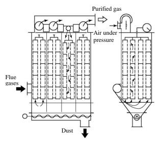
Fig. 1.31. Multi-chamber bag filter with supply of the dusty flow into the bags
