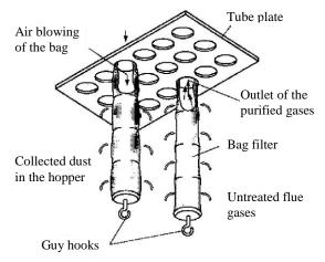
Fig. 1.30. Design and function of fabric bag filter with supply of the dusty flow from periphery to the bag
