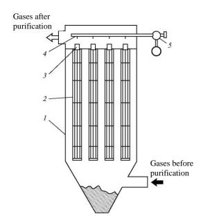
Fig. 1.32. Fabric bag filter with supply of the gas flow outside the bags and with one-side pulsed blowing:
