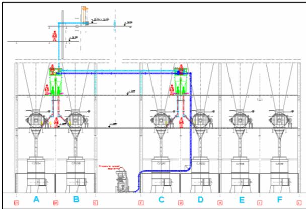
Fig. 2. Ash conveying pipe route
