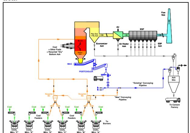
Fig. 1. The Magaldi Ash Recycling system flow-diagram
