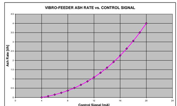
Fig. 4. Vibrofeeder ash rate vs. Control signal
