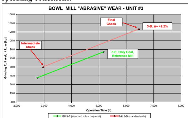
Fig. 5. Bowl mill abrasive wear results
