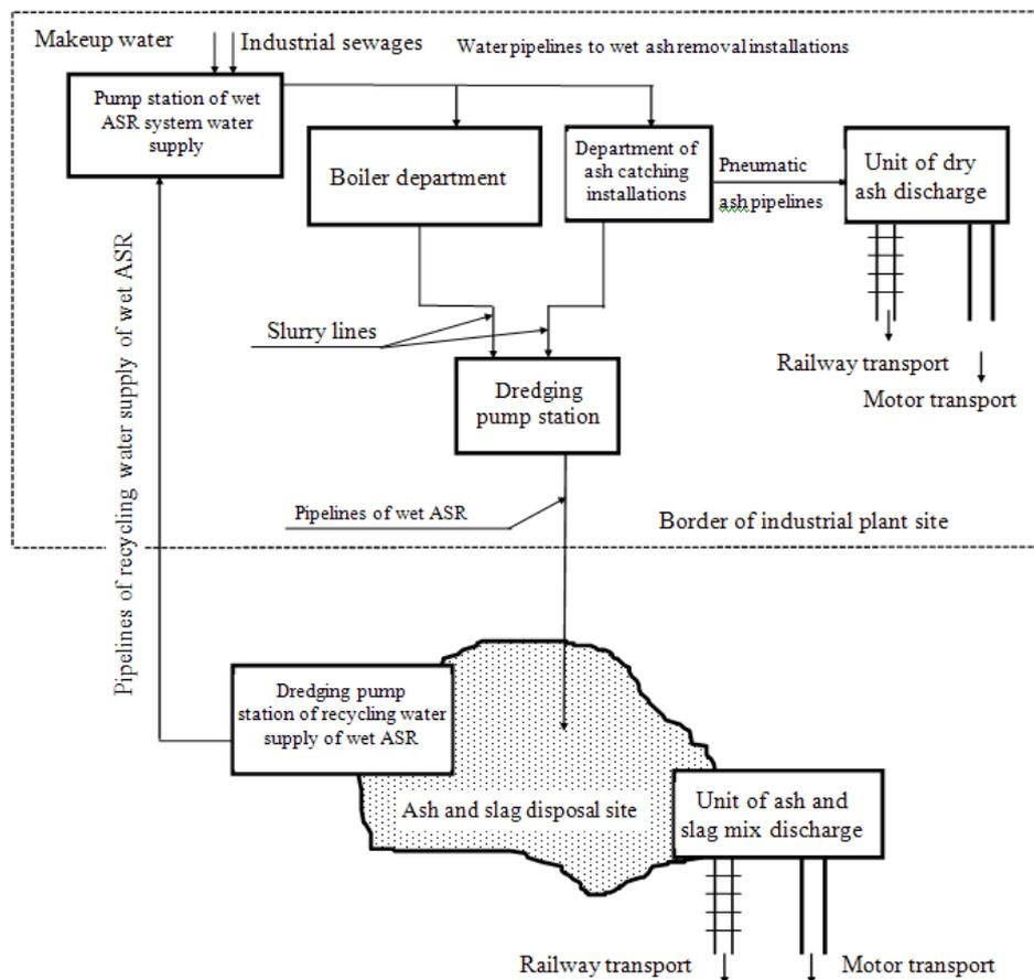
**Fig. 3. Block diagram of the combined ash and slag removal system with shipment of ash to the customer from the unit of dry ash discharge and ash and slag mix from the disposal site.**
