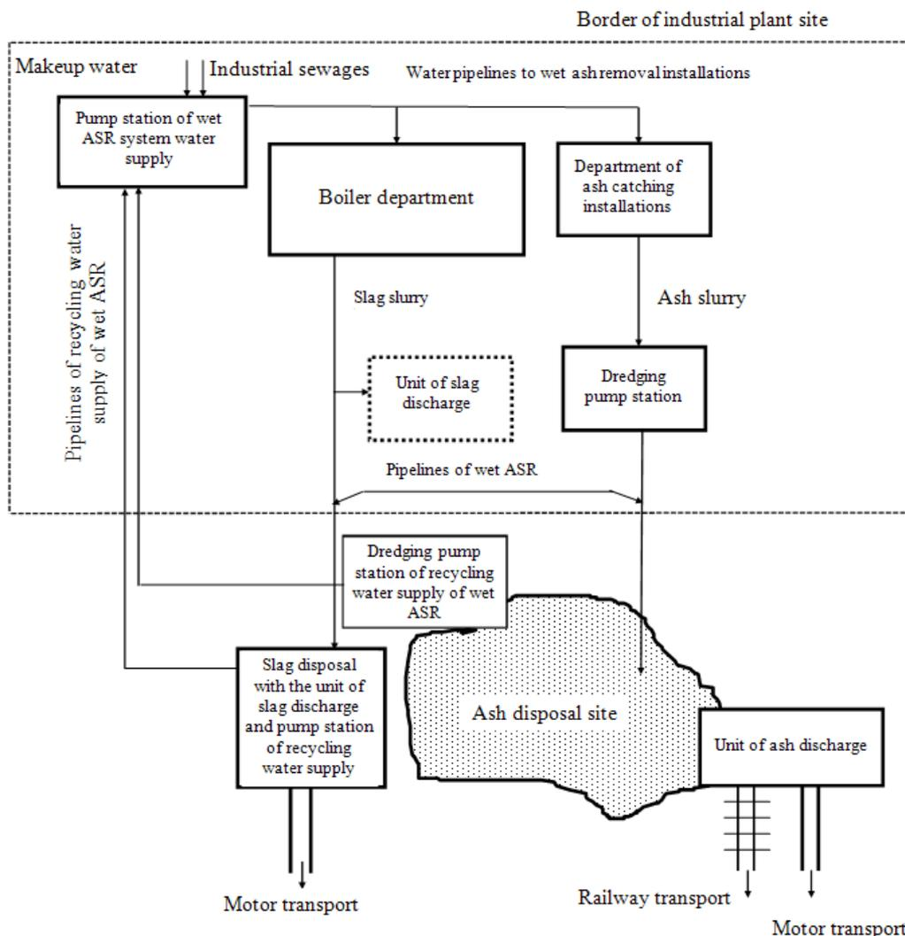
Fig. 2. Block diagram of wet ASR system with separate removal, landfilling and discharge of ash and slag.
