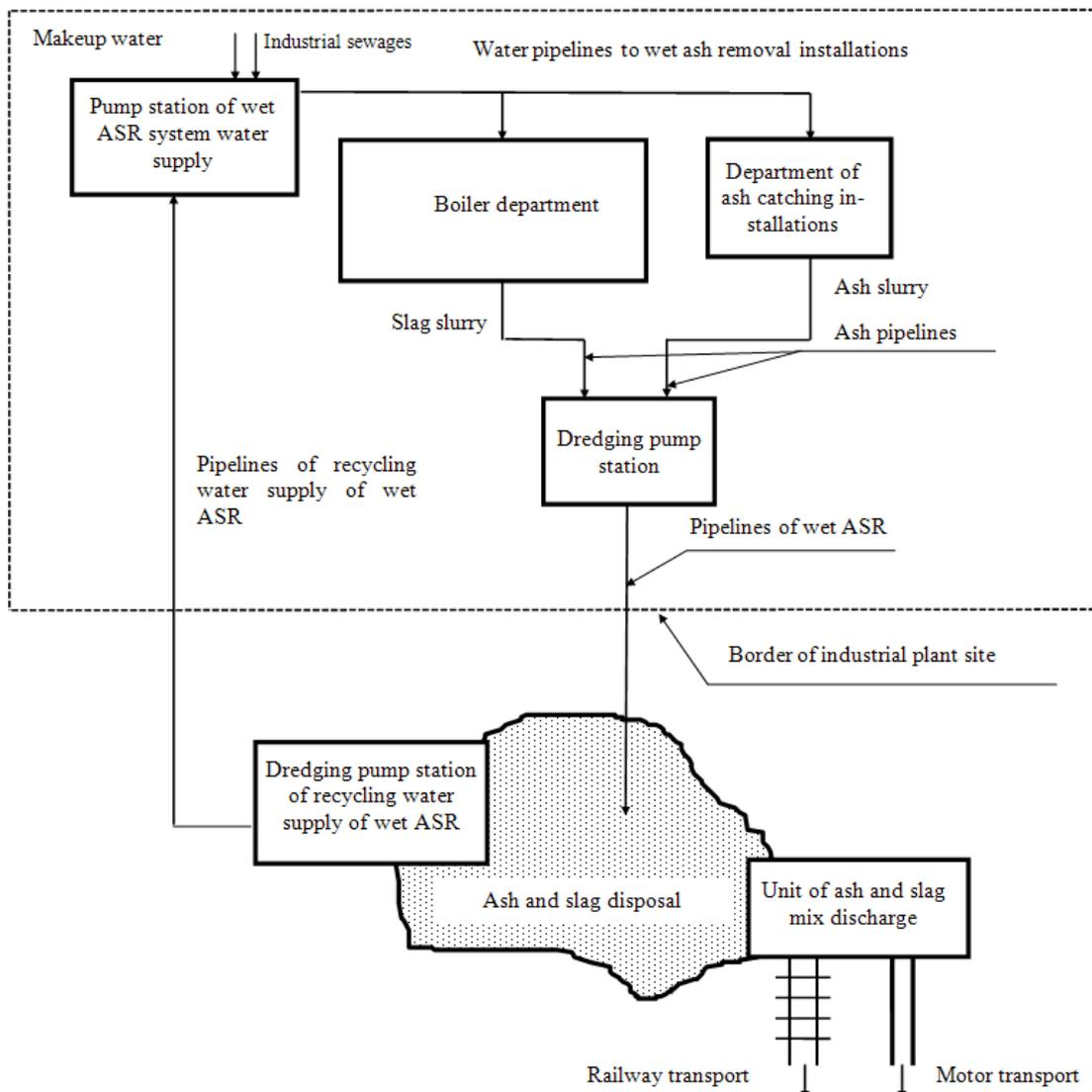
**Fig. 1. Block diagram of traditional wet ASR system at TPPs at combined ash and slag conveying to the disposal site and discharge of ash and slag mix from the completed sections of disposal site to the motor and railway transport.**
