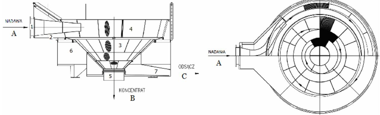
Fig. 1. Centrifugal dewatering sieve-OSO: A – feed material; B –concentrate; C –drain-off; 1 –nozzle outbox; 2 –steering wheel casing; 3 – conical sieve basket; 4 –steering wheel ; 5 –dewatered product exit; 6 –drain-off cumulative vessel; 7 – drain-off exitumtion.
