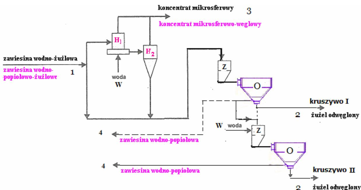
Fig. 3. Production of slag aggregates, coal concentrates, and cenospheres – a diagram
