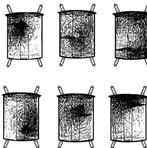
**Fig. 1.84. A nature of mixing in the furnace section of jets, flowing from tertiary blast nozzles of the front and back walls of the furnace of BKZ-210-140F boiler**
