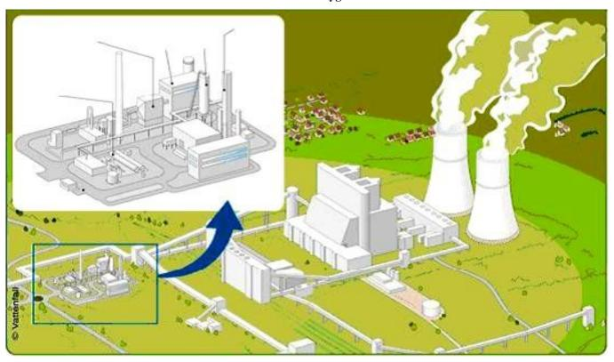
Pilot installation of Vattenfall of 30MW at TPP Schwarze Pumpe (brown coal) Put into operation in September, 2008. Output of  $CO_2$  is 10 t/h. Cost - more than 100 million US \$. Purpose of the project is investigating a concept of the unit of 250-350 MW for its construction in 2015-2020.
