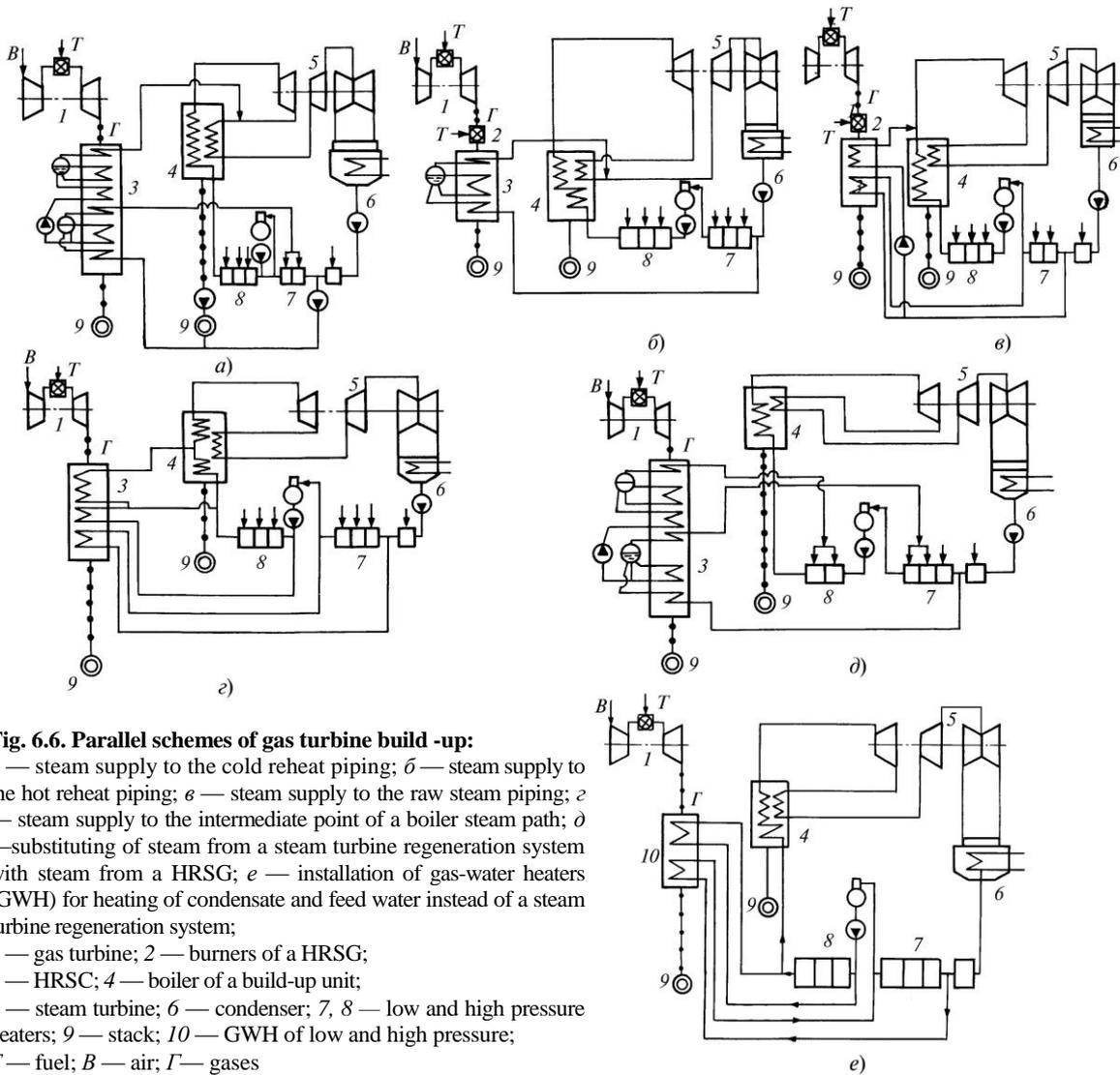
**Fig. 6.6. Parallel schemes of gas turbine build-up:**
