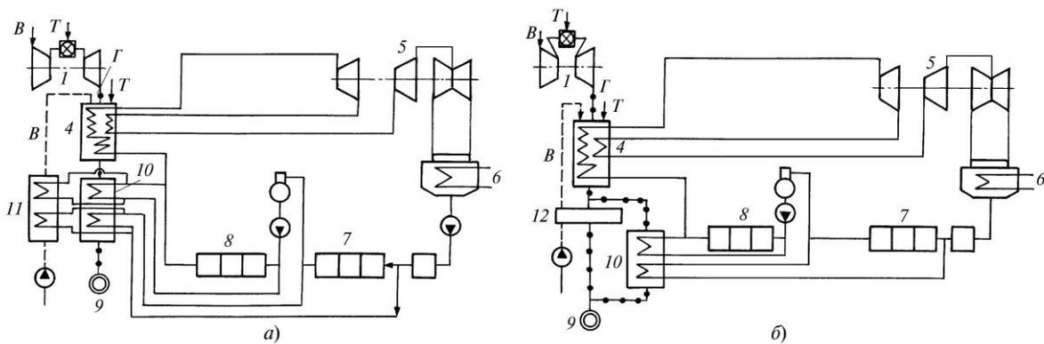
**Fig. 6.7. Discharge schemes of gas turbine build-up:**
