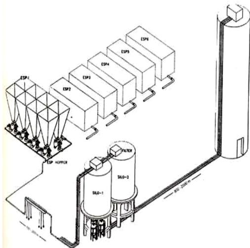
Fig. 6. Typical Dry Fly Ash Handling Arrangement at a Power Station
