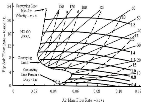
Fig. 4. Conveying Characteristics for Fine Grade of Fly Ash with Conveying Line Inlet Air Velocity Data Superimposed
