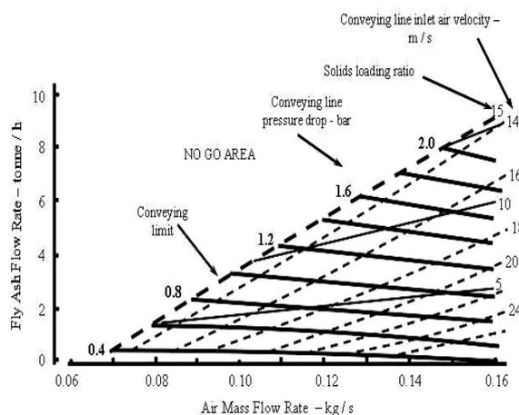
Fig. 5. Conveying Characteristics for Coarse Grade of Fly Ash with Conveying Line Inlet Air Velocity Data Superimposed
