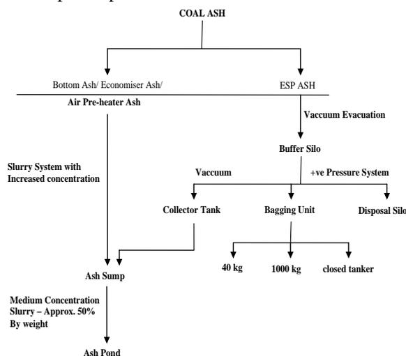
Fig. 7. Recommended Options for Coal Ash Handling and Safe Disposal
