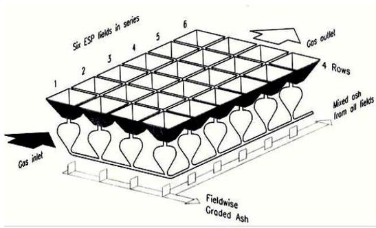
Fig. 2. Typical Arrangement of Electrostatic Precipitator Ash Collection Hoppers
