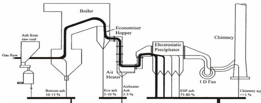
Fig. 1. Ash Accumulation Points and Typical Ash Distribution of a Dry Bottom Furnace
