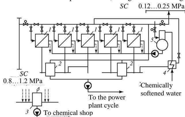
**Fig. 2.4. Multi-stage evaporation unit at an industrial-heating thermal power plant:** 1 — vaporizer; 2 — distilled water expansion tank; 3 — blow-off water expansion tank; 4 — chemically softened water heater; 5 — deaerator; SC - steam collector
