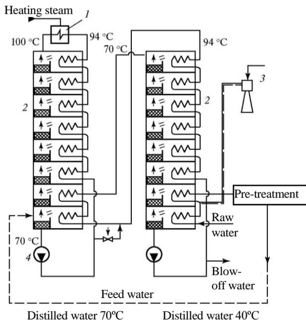
**Fig. 2.6. Flash type vaporizer IMB-50:** 1 — main heater; 2 — vaporizer; 3 — ejector; 4 — circulation pump
