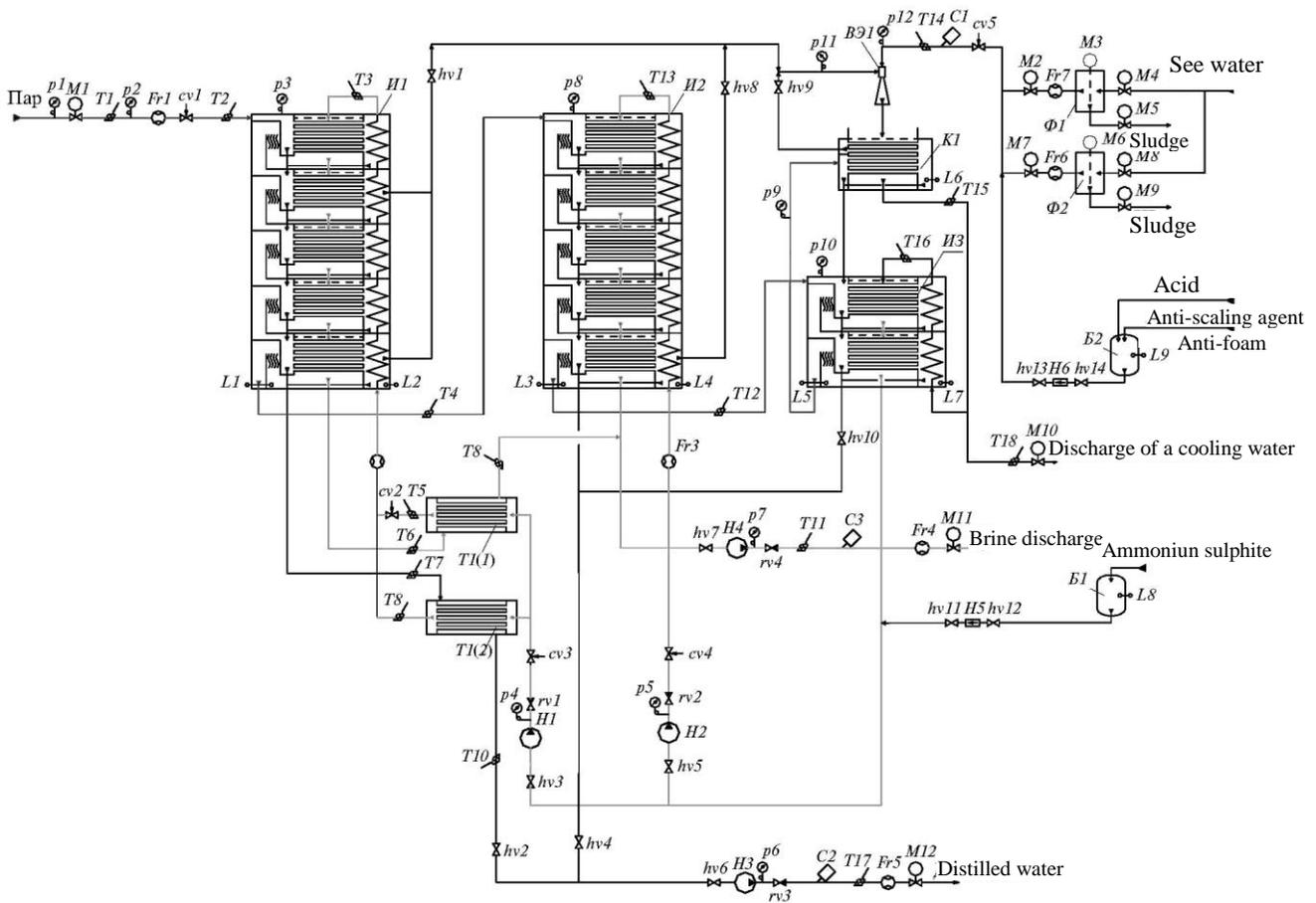
**Fig. 2.5. Distillation-desalination unit with horizontal tube film apparatus:**
