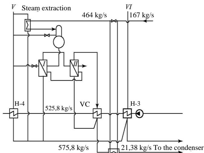
**Fig. 2.3. Modular evaporation unit in a condense power unit scheme:** H- heater; VC- vaporizer condenser
