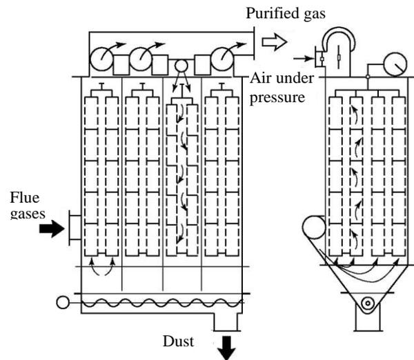
**Fig. 1.31. Multi-chamber bag filter with supply of the dusty flow into the bags**
